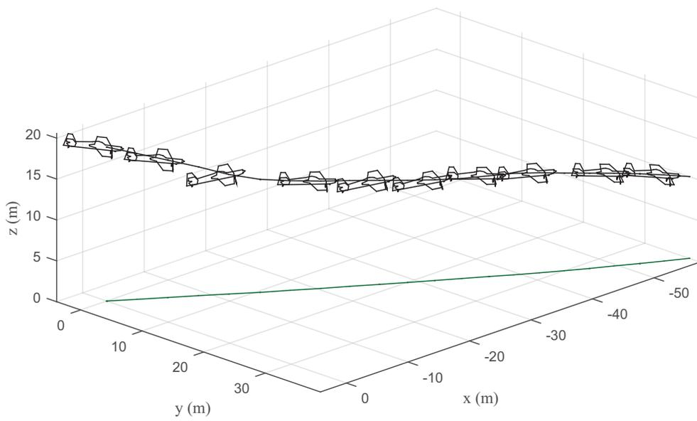
**Figure 9. Trajectory of the aircraft during up elevator response.**
