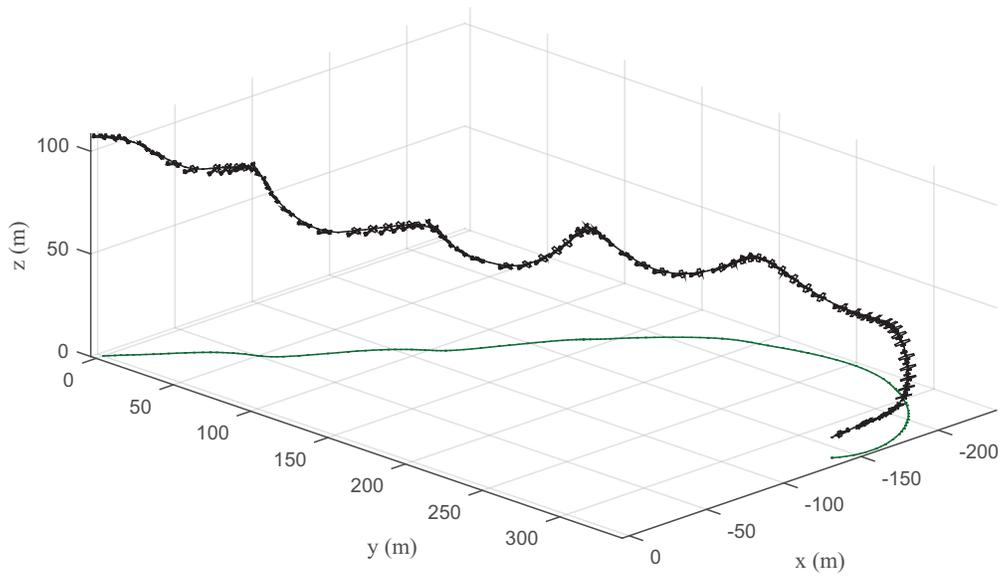
**Figure 17. Trajectory of the aircraft during phugoid with full flaps.**
