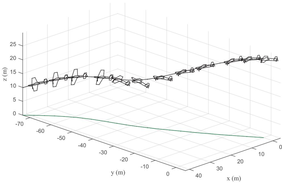
**Figure 21. Trajectory of the aircraft during stall with full flap.**
