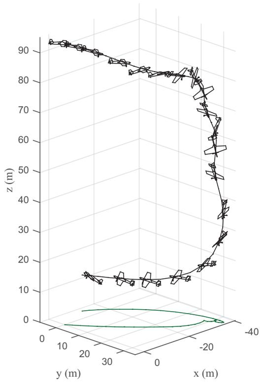
Figure 35. Trajectory of the aircraft during spin with full flap.
