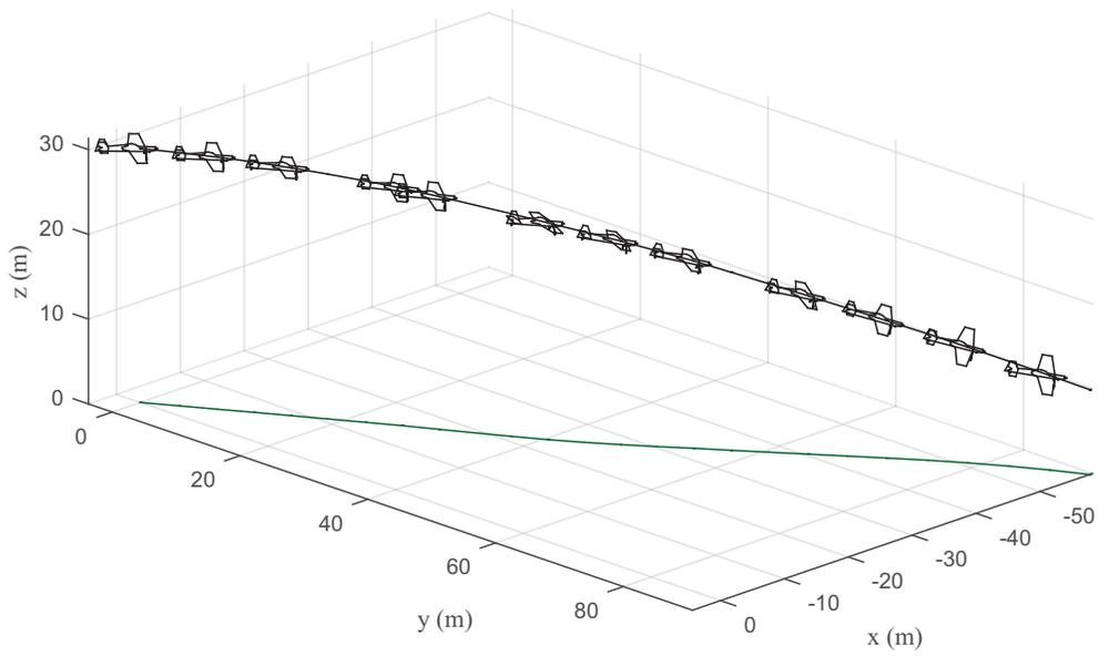
Figure 29. Trajectory of the aircraft with left and right rudder inputs.
