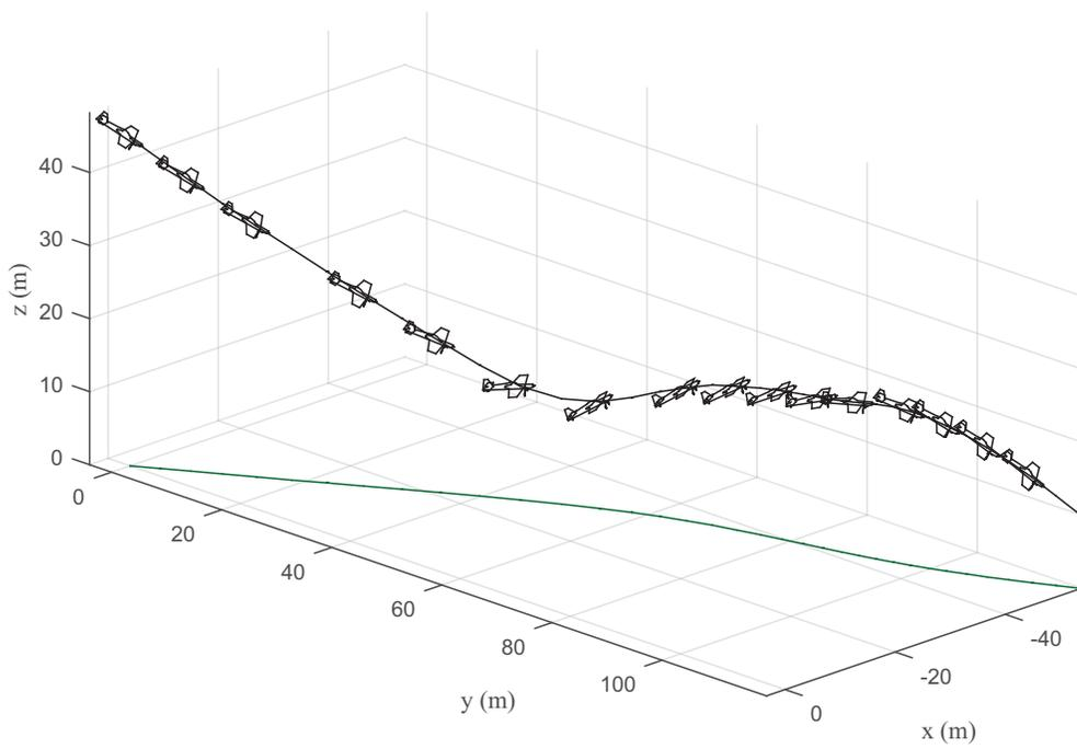
**Figure 19. Trajectory of the aircraft during stall with zero flap.**
