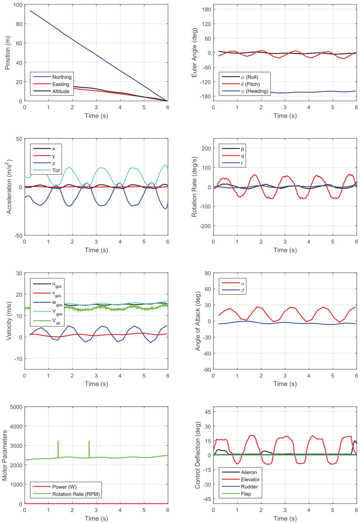
Figure 12. Time history of aircraft state during up and down elevator response.
