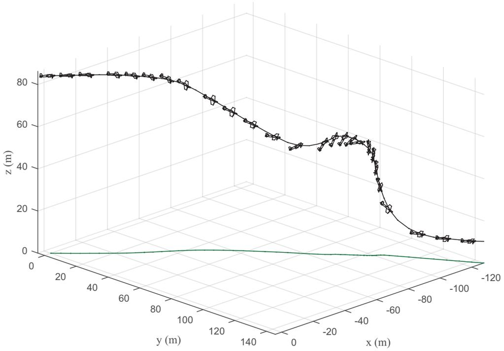
**Figure 23. Trajectory of the aircraft during deep stall with zero flap.**
