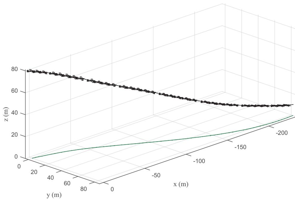
**Figure 7. Trajectory of the aircraft during idle decent with half flaps.**
