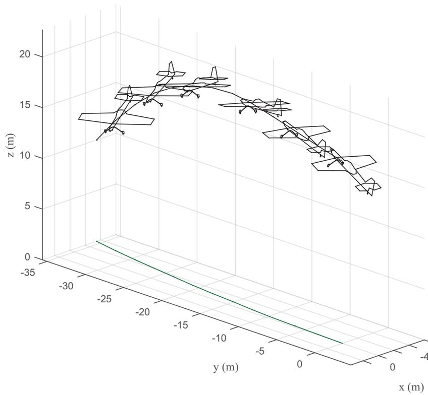
**Figure 11. Trajectory of the aircraft during down elevator response.**
