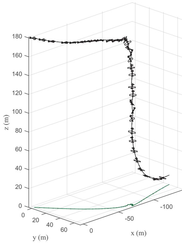
**Figure 33. Trajectory of the aircraft during during spin with zero flap.**
