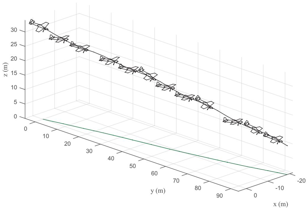
Figure 13. Trajectory of the aircraft during up and down elevator response.
