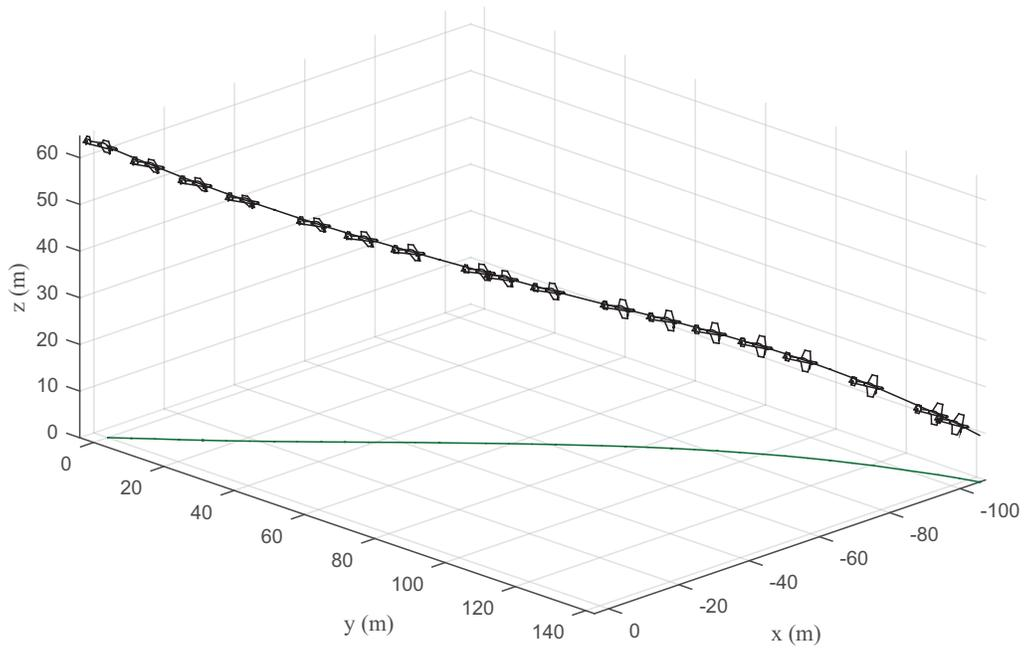
**Figure 5. Trajectory of the aircraft during idle decent with no flaps.**
