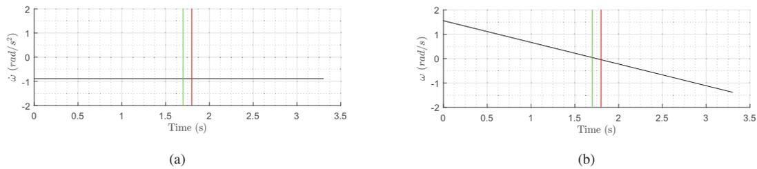
**Figure 1.** A example moment of inertia test where data is collected about zero angular velocity, starting at the green line and ending at the red line with: (a) a constant angular acceleration of  $-1$  rad/s and (b) a perturbed initial velocity of  $1.5$  rad/s.
