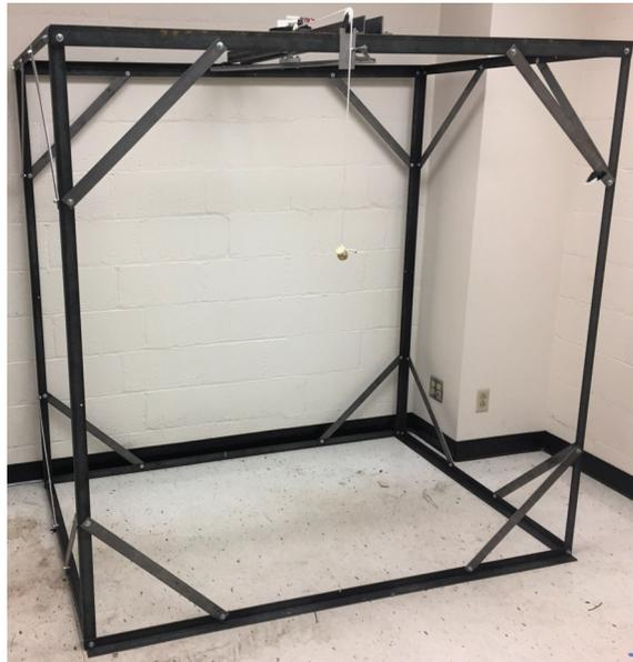
Figure 2. Moment of inertia measurement rig
