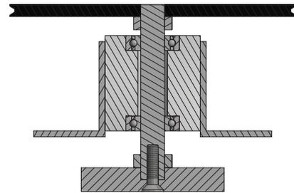
Figure 5. Cross section of rotation assembly.
