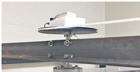
Figure 6. Moment of inertia measurement rig instrumentation.
