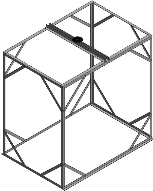
Figure 4. CAD drawing of the moment of inertia testing rig.
